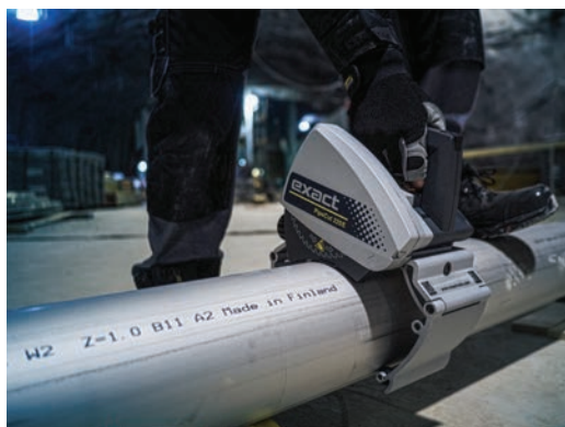
Cutting stainless steel pipe
