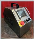
Speed, torque and current are controlled and displayed during complete cutting and beveling process.
